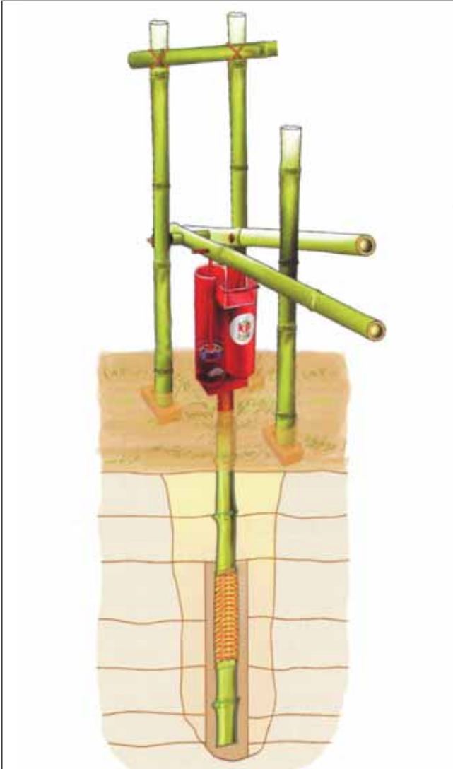
Classical bamboo treadle pump, which can lift water up to 6 m
