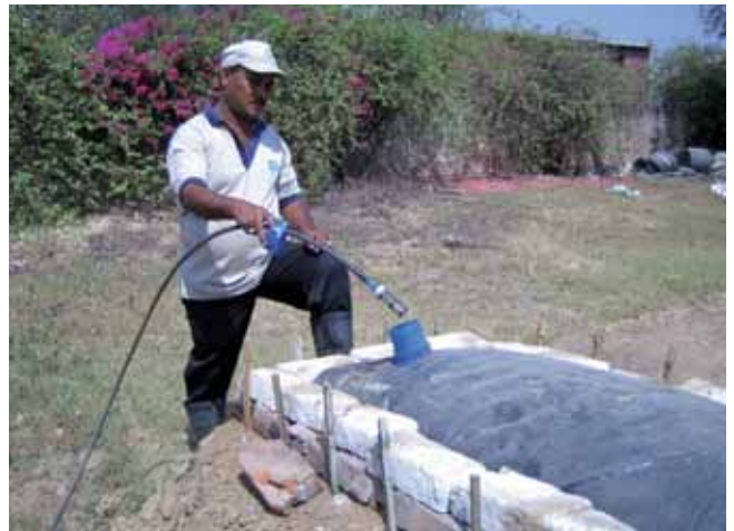
New low-cost water tanks are developed and tested. They can produce enough pressure to operate drip irrigation systems
