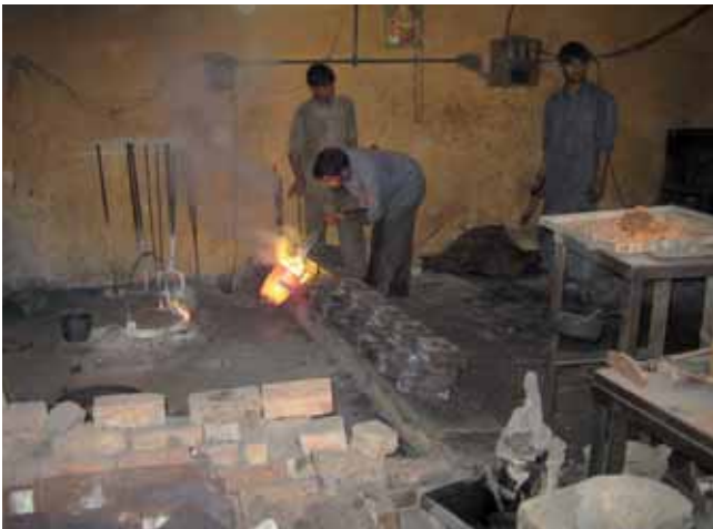
The new sprinkler heads manufactured in this foundry in India are made of brass; they can be produced locally
