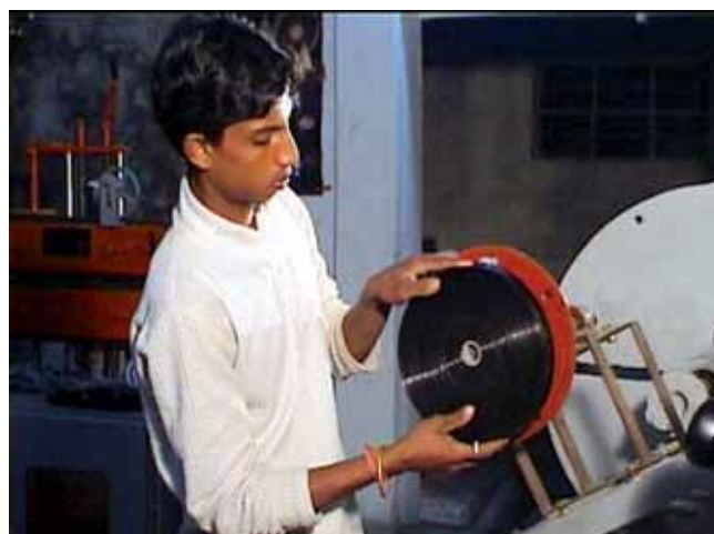
The same machine used by local manufacturers to produce tube for 'Pepcee' packaging can be used for 'KB Drip', sold in rolls by the kilogram
