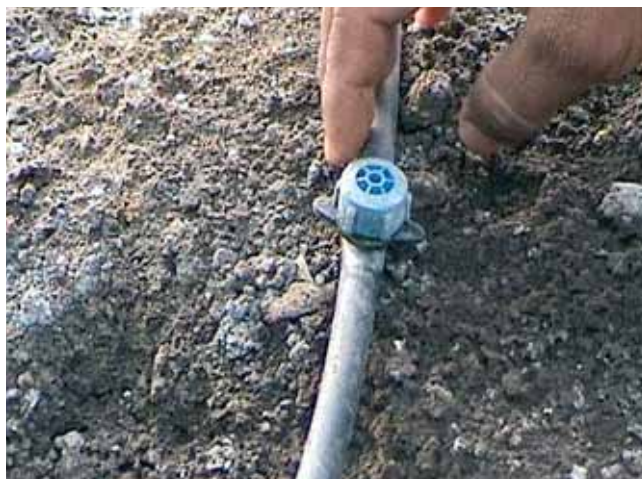
Such a BIS standard dripper costs Rs2.5. Farmers dislike it – it is very expensive and often clogs
