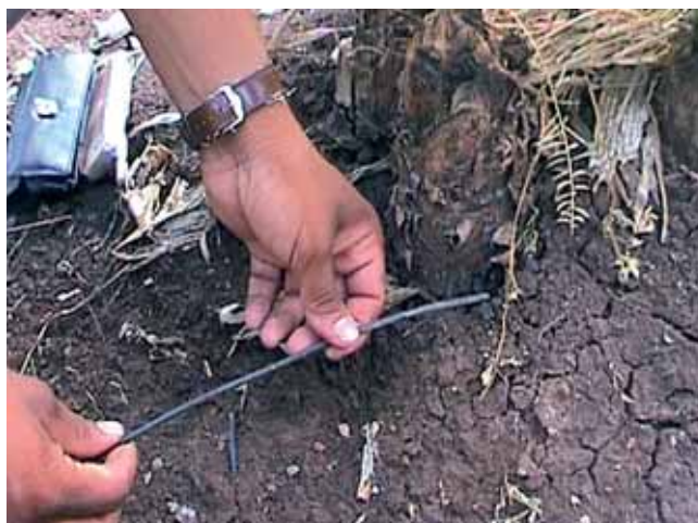
These micro-tube emitters cost ten times less and do not clog easily. But government subsidies are only available for systems with BIS standard drippers
